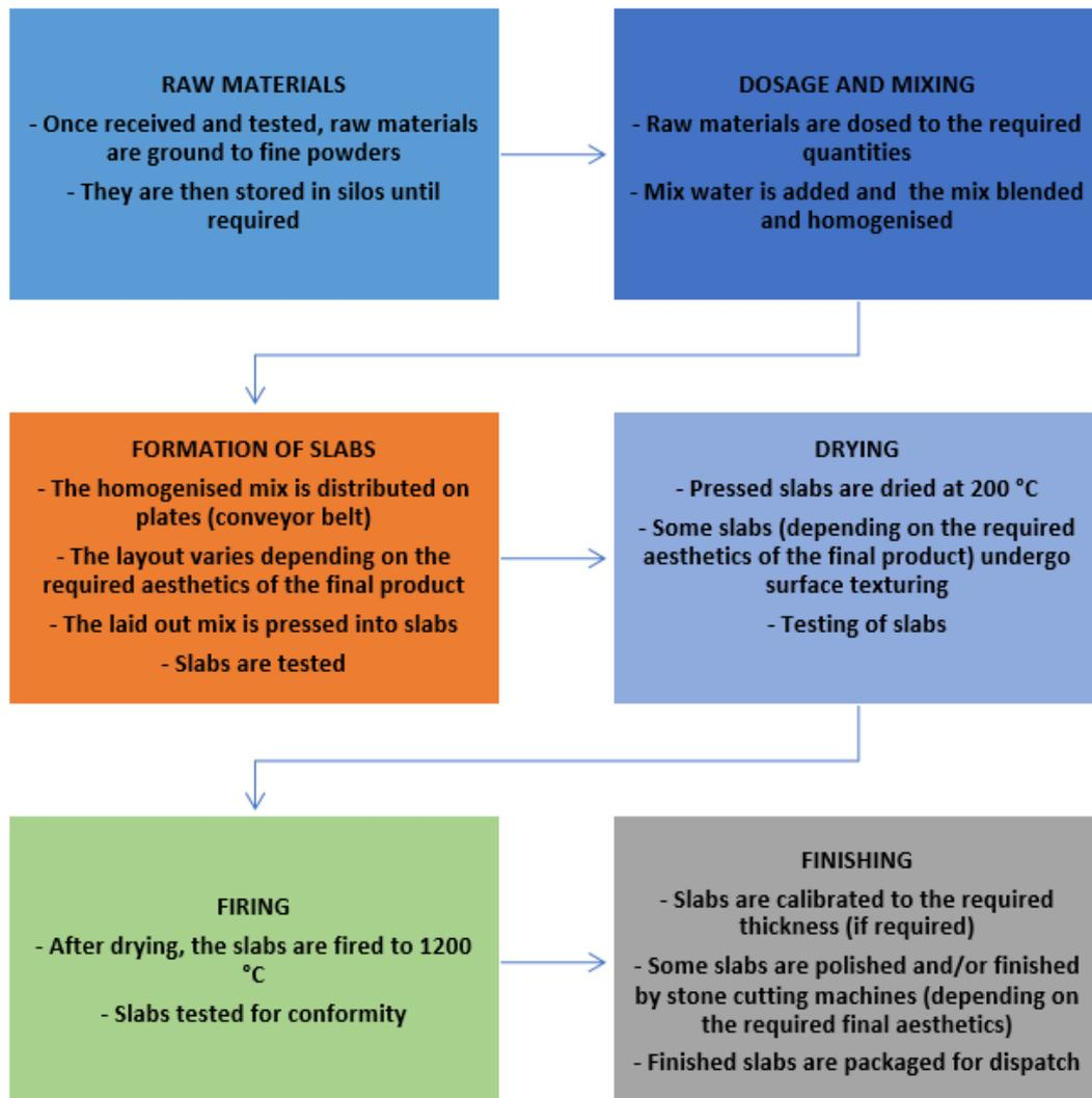
**Figure 1:** Typical process flow for the manufacture of Lapitec sintered stone slabs products, provided by Lapitec SpA.
